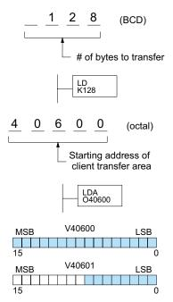
For an RX instruction, the CPU reads the number of bytes previously specified from the server, placing the received data into its memory area beginning at the LDA address specified.
