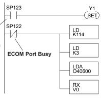
The "Port Communication Error" bit turns on when the PLC has detected an error. Use of this bit is optional. When used, it should be ahead of any network instruction boxes since it will be reset when an RX or WX instruction is executed.
